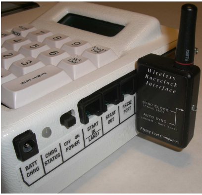
For Clock Control/Synchronization (or Both Finish Results & Clock with TM modification)
