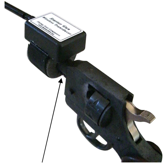
Barrel of Starting Pistol inserted into foam "Barrel Sleeve"
